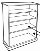
Shelf and side panel Note: the shelves are glued in place
